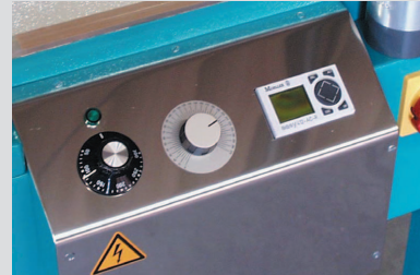
Operation panel with thermostat, speed control of conveyor belt and a digital display and control of sealing time
